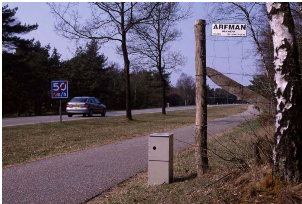
Figure 51. An animal detection system (infrared break-the-beam system manufactured by Calonder Energy, Switzerland) at a gap in a wildlife fence near ‘t Harde, The Netherlands (© Marcel Huijser).
