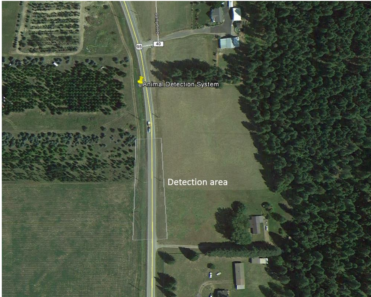
Figure 3. The Location of the Doppler Radar System and the Detection Area.
