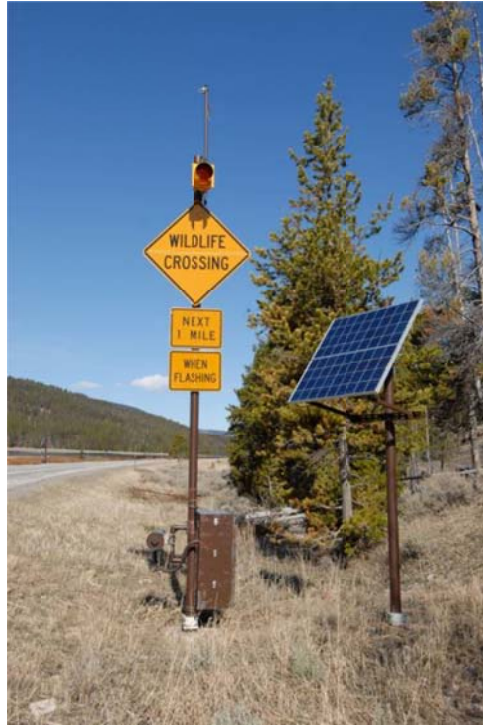
Figure 30. An animal detection system (microwave radio signal break-the-beam system manufactured by Sensor Technologies & Systems, Scottsdale, AZ) installed along a 1 mile (1,609 m) section of US Hwy 191 between Big Sky and West Yellowstone in Yellowstone National Park (© Marcel Huijser).
